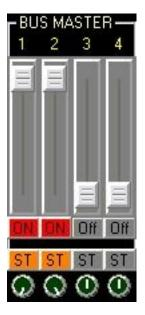
An exception to what said before is that the 4 pan of Bus Master in the Yamaha can be controlled through the wheel "Parameter" in the page. 3 of Pan / Routing ", in software rather have 4 separate rotary controls in its routing switches to the Stereo Bus (**ST**ST).
