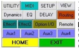
To switch between channels 1-16 to optional ones 17-24 press, in transmit mode, the button **Option I/O** it remark its activity becoming **Option I/O** and pointing with <u>yellow text on black background</u> channels labels **17-24** on bottom of the window. To return to manage the channels 1-16 you press the button **HOME** that things will reverse again. They are, as the Yamaha of course alternative, and I repeat, being impossible receive the corresponding messages of the Yamaha is
