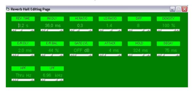
The window that appears when you press the button **EDIT**, somewhat reminiscent of the display of the Yamaha, but it condenses the parameters in a single screen (instead of the two or three in the Mixer). Parameters can be edited easily through the thin sliders (In the usual way of the software). In real-time MIDI messages change the settings of the Yamaha.
